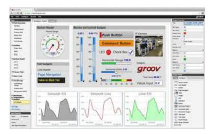
Prior attempts to mimic operator interface screens in a browser have been poor, Hougland explained, with limited scalability. This system uses HTML5 to scale graphics, buttons, labels, images, live video, trends – everything – to the screen size. The only software needed is a browser. On the development page for the software, another tab allows tweaking or reordering to optimize gadget location with screen shape, but scaling works fine, even without changes, as a demonstration showed.
