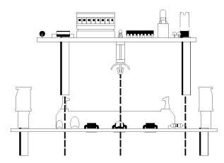
If you are attaching a B100 to a G4PB16L mounting rack, you must first attach a plastic, removable standoff to the brain board as shown in the figure above. Continue by installing the brain board to the mounting rack as described above and as shown in the figure to the left.
