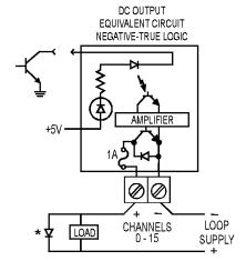
\*Note: Commutation diode must be used on inductive loads. Typically, use diode 1N4005
